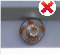
Fixed using galvanized screw with bonded galvanized washer
